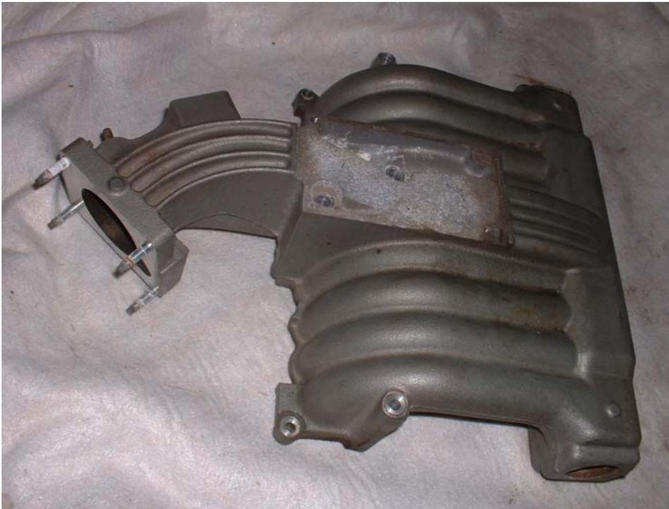
1994-95 Mustangs and 1991-93 Thunderbirds have the lowest intake profile at 9.5 inches, but to keep the intake runner length the intake is wider and contacts the master cylinder. Those intakes mount the throttle body at a 45° angle aimed towards the back of the headlight, so if the upper intake is flipped to the driver's side, the throttle body aims directly towards the brake master cylinder.
