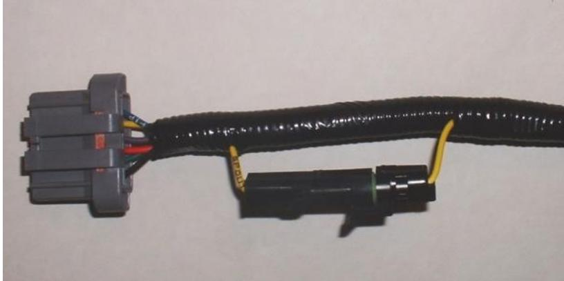
To set the base timing you need to disconnect the SPOUT connector, which is near the distributor. This cuts off communication from the computer and allows you to set the base timing. Lots of people preach “set it higher for more power,” DON'T! The computer just woke up, and is now learning about all the performance parts you added to the mix. The stock 10° setting is all you need for now. Once the light is flashing on 10° BTDC put the SPOUT connector back in and tighten the distributor.
